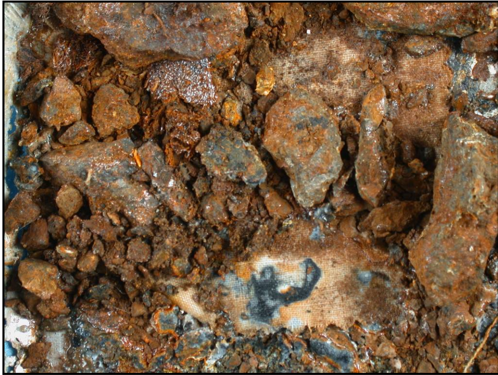
Figure 7: Modern Textiles in Simulated Concretion Environment
