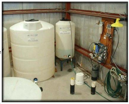
to water purified by reverse-osmosis (RO water). Over time, the salts present in the objects move out into the desalination baths, leaving the artifacts as free of salts as possible.
